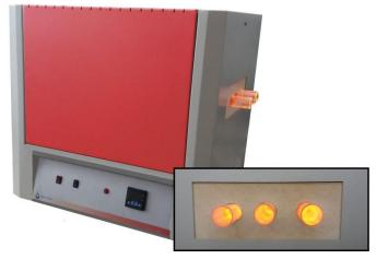
**Kare Series** tube furnaces are single zone controlled furnaces up to  $1300^{\circ}$ C. The tubes of this furnaces are independed from heating elements and can be easily replaced by the operator. The heating zone can be produce between 200 mm – 450 mm. The tubes can used ceramic and quartz.
