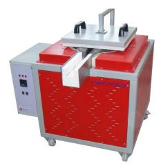
The custom design **PID control** devices produced for the our company, minimizes the heat fluctuations on the set values. Every step on the control devices can be defined up to **9999** minutes and in case of a power loss the system resumes on.
